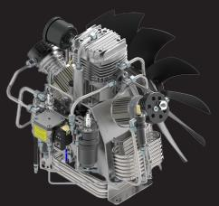
The bearings of the crankshaft have rollers, extremely robust and made in Europe which guarantee a long life of the compressor. An oil pump provides a constant lubrication of the inner workings of the block with oil cleaned of impurities by a filter and by a magnet which catches any metals present in the lubricating oil. The compressed air cooling is obtained by inter-stage stainless steel cooling coils.
